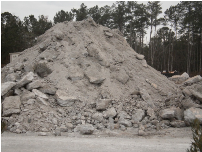
Photo Coal ash pile used for road build-up Photo courtesy of Steve Johnson
