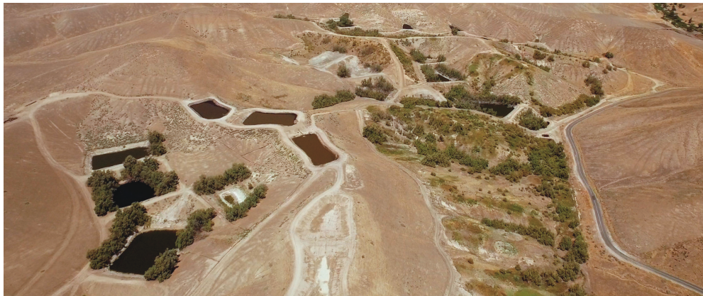
Aerial Photo of the Racetrack Hill pit facility, East of Bakersfield. The 27 unlined pits and spray fields (green hillside in photo) have dispersed contaminants to the underlying groundwater, which supplies drinking water and irrigation for neighboring communities.
